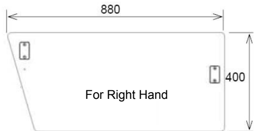
Fig.11 Arm support (carbon)(Option)
