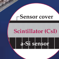
Cutaway diagram of a-Si Flat Panel Detector layers
